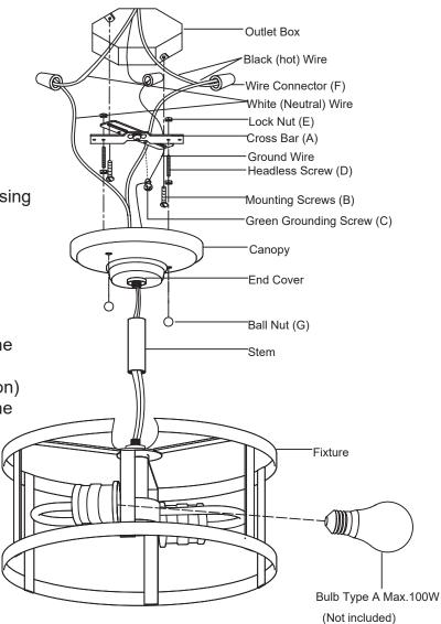
5. Attach the canopy to the cross bar by inserting two headless screws, and then secure it with ball nuts.
