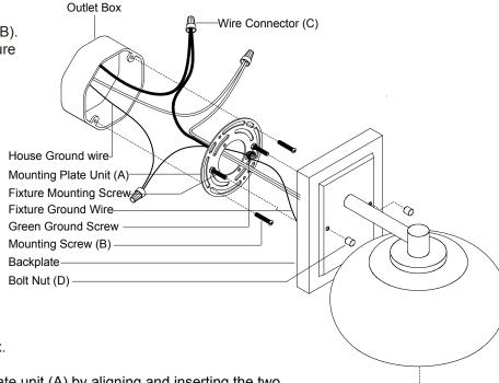
3. Attach the backplate to the mounting plate unit (A) by aligning and inserting the two fixture mounting screws from the mounting plate unit (A) into the open holes on the backplate, then expose fixture mounting screws before screwing the two bolt nuts (D).
