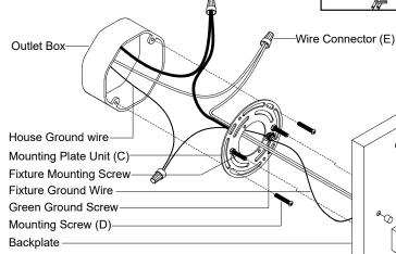
4. Attach mounting plate unit (C) to the outlet box using two mounting screws (D). Adjust the length of the preinstalled fixture mounting screws if necessary.
